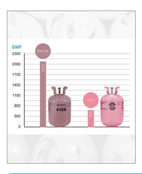
With a GWP of 675, R-32 contributes less to global warming potential compared to other refrigerants like R-410A. Because of R-32's excellent thermodynamic performance characteristics, an R-32 system could have up to 40% less charge than R-410A in certain applications, meaning you could reduce refrigerant usage in the equipment and potentially also reduce quantities leaking to the environment.
